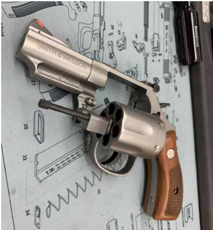
Note new ball-detent lock up which allows for full length ejector rod, giving more reliable ejection.
